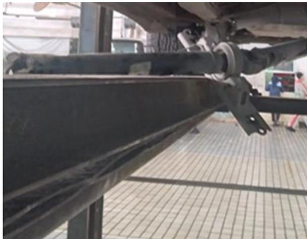
**Gambar 4. Poros Propeller**
